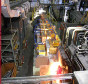
Hot Former Heater
