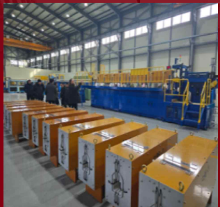
1800kW Square Billet Heater
