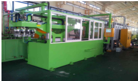
250kW Pin/Bushing Heater
