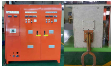
160kW BUILD-UP Heater for Welding
